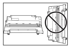
4 Place the drum unit flat on a clean, level surface.
