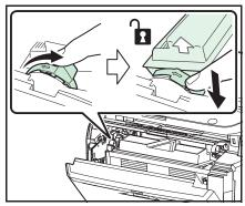
2 Turn the toner container lock lever to the unlock position. Push the toner container lock lever to the position marked by the arrow and pull out the toner container.
