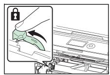
**6** Turn the toner container lock lever to the lock position.
