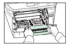
**3** Remove the drum unit from the machine by holding the green levers with both hands.
