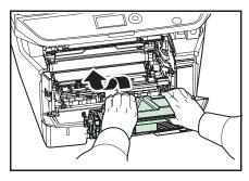
**8** Return the developer unit to its position, aligning the guides at both ends with the slots in the machine. Then, close the front cover.
