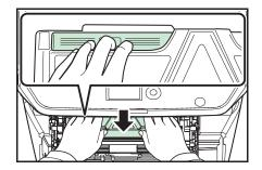
Install the new toner container in the machine. Push firmly on the top of the container at the positions marked PUSH, until you hear a click.
