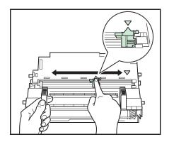
6 On the drum unit, slide the main charger cleaner (green) back and forth 2 or 3 times to clean the charger wire, then return it to its original position (CLEANER HOME POSITION).
