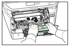
2 Lift the developer unit together with the toner container out of the machine.
