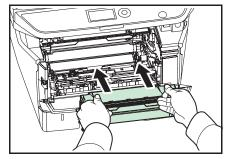
7 When cleaning is complete, return the drum unit to the original position.
