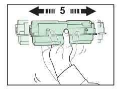
3 Take the new toner container out of the toner kit. Shake the new toner container at least 5 times as shown in the figure in order to distribute the toner evenly inside the container.
