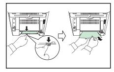
Open the duplexer's cover at the rear of the machine and remove any jammed paper.
