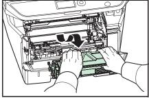
Open the front cover, and lift the developer unit together with the toner container out of the machine.
