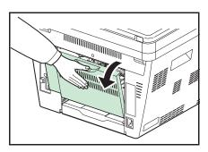
1 Open the rear cover and remove the jammed paper by pulling it out.
