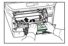
6 Insert the developer unit together with the toner container, back into the machine. Close the front cover. The machine warms up and resumes printing.
