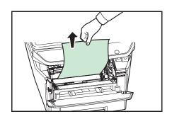
4 If the jammed paper appears to be pinched by rollers, pull it along the normal running direction of the paper.
