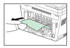
If the paper is jammed inside the fuser unit, open the fuser cover and remove the paper by pulling it out.
