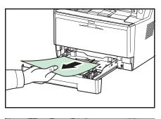
1 Pull the paper cassette all the way out of the machine. Remove any partially fed paper.
