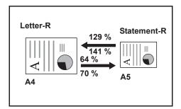
Automatically reduces or enlarges the original image suitably to the selected paper size.
