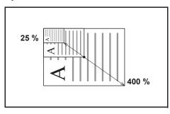
Manually reduces or enlarges the original image in 1% increments between 25% and 400%.
