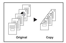
Produces two-sided copies from one-sided originals. In case of an odd number of originals, the back side of the last copy will be blank.
